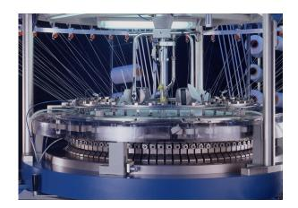
Traditional Orizio modular frame, renovated in its functionality robustness and aesthetics, with the new, integrated control panel which allows the fruition of new technologies and completes the machine's control, the needles selection and the following functions:
